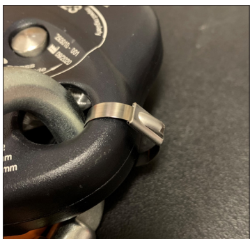
Abb.1 Cable tie at the LORY/ Kabelbinder am LORY
