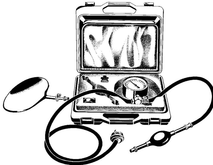
Inflate the dummy head with approx. 70 pump strokes and close with tube clamp. Afterwards connect pump ball with suction side to leak tester.
